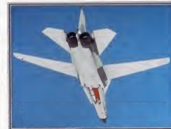
▲ Weapons bay The internal weapons bay could be used for either extra fuel or short-range nuclear missiles.
